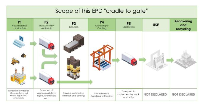
The following diagrams, designed for this EPD using Air.e LCA software, show the materials, fuels consumption, energy consumption transports and other procedures included in the assessment.
